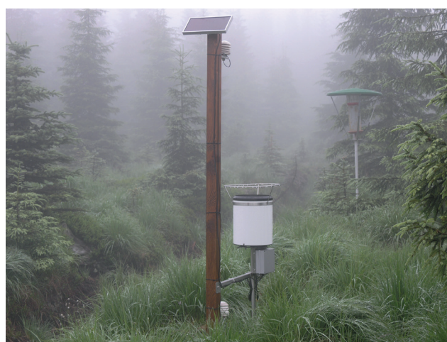
Fig. 1 Fog samplers: (a) active fog sampler, Sum_CH, (b) passive fog sampler, KrK_SH and (c) passive fog sampler in the background with rain sampler in the foreground, Jiz_CN, photographer: M. Tesař.
